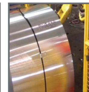
Data Matrix marking on Aluminum Coil
